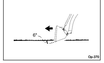
With bucket level, start a cut at notch approximately 2 inches deep. Hold depth by feathering bucket control to adjust cutting lip up or down. When front tires enter the notch, adjust lift cylinder to maintain proper depth.
